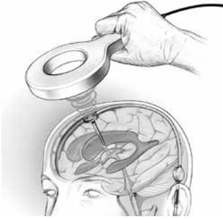
Fig.4: Pressure measurement with the Reader Unit of the SENSOR RESERVOIR/ SENSOR PRECHAMBER
